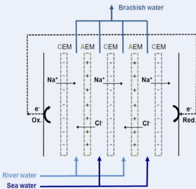
Fig 1. Simplified principle of RED.
