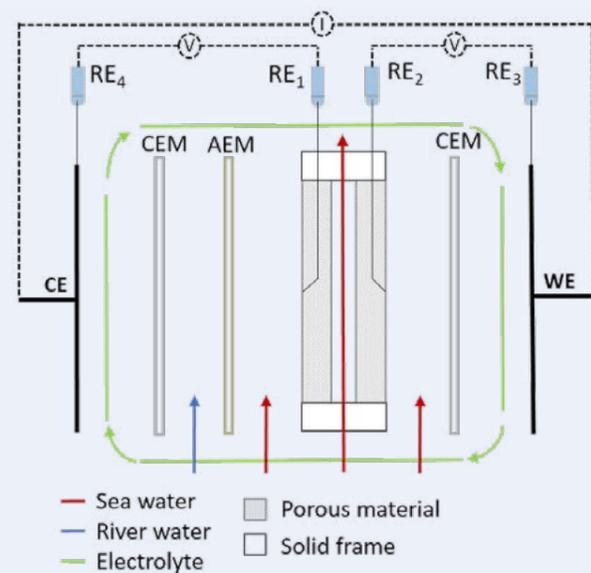
Fig 3. Schematic illustration of fouling monitor. Adapted from [3]
