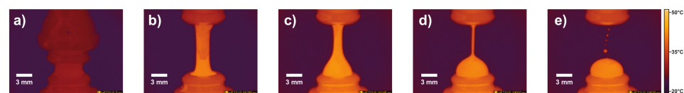
Figure 9. Thermographic images of a vertical water bridge from ignition to extinction. Representative series of long-wave infrared (7.5-9.0 \mu\text{m} ) images characterizing the operational stages for vertical liquid bridges shown for water: (a) ignition, (b) expansion, (c) reduced voltage, (d) ligand formation, (e) breakup into droplets under the influence of rayleigh-plateau instabilities. Elapsed time is shown in msec. The background contrast was adjusted in the last frames to enhance droplet visualization. Stills from supplemental video S7. Please click here to view a larger version of this figure.
