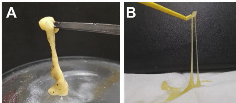
**Fig. 1.** (A, B) - Viscous sludge produced from freshwater-MBR at COD/N ratio 60 (A) and 100 (B). (C) - Soluble-EPS viscosity as a function of shear rate at room temperature (21 °C). (D) - Soluble-EPS concentration versus viscosity at a shear rate of 12.2 s<sup>-1</sup>. Viscosity of the influent was obtained at a shear rate of 244.8 s<sup>-1</sup>. Sal S-EPS: saline soluble-EPS, FW S-EPS: freshwater soluble-EPS.
