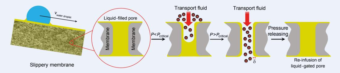
Fig 1. Schematic illustration of SLIM and gating mechanism of adaptive pores (from left to right). In this figure,  $\delta$  is the liquid film thickness lining the pore and  $P_{critical}$  is the pressure required to open up the liquid-filled pore.
