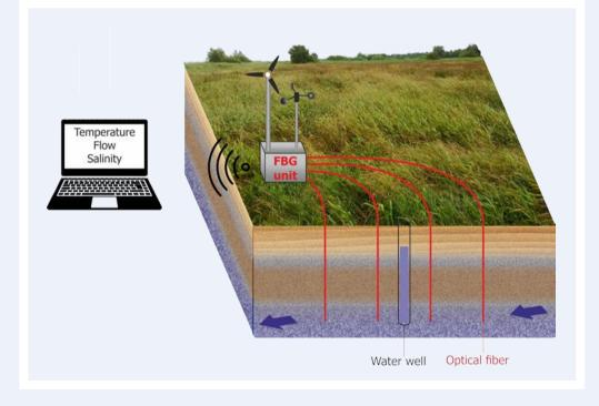
Fig. 1: FBG sensors gathering information about subsurface flow, temperature and salinity in order to identify source and quality of drinking water
