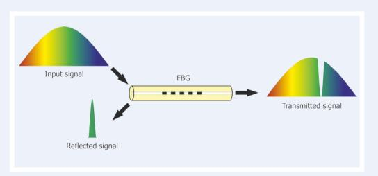
Fig. 2: Fiber Bragg grating reflecting narrow part of input spectrum
