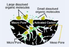
Figure 1 Activated carbon pore structure and adsorption sites [4].
