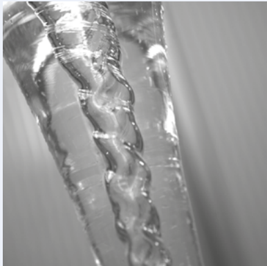
Fig 1. High speed camera image of air-water interface in hyperbolic funnel
