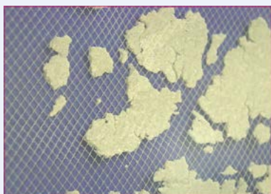
Figure 3. Membrane scaling (www.impomag.com)
