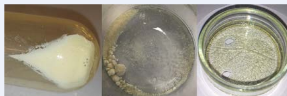
Figure 2. CGP after extraction. Left: After centrifugation, Center: Lyophilized, Right: After 24 h at 105^\circ\text{C} .
