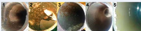
Figure 1: Biofilm growth on different pipe materials, 1 – ductile cast iron pipe, 2 – gray cast iron pipe, 3 – galvanized steel pipe, 4 – stainless steel clad pipe, 5 – polyvinyl chloride (adapted from [1])
