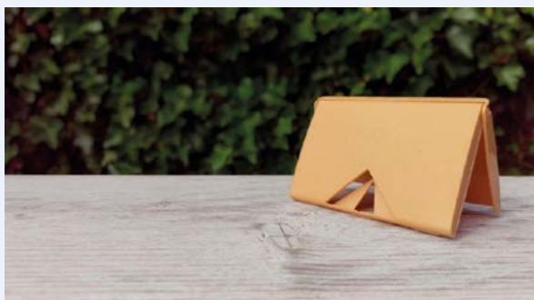
Fig 1. Business card holder made during the PHARIO project using municipal activated sludge [1] .
