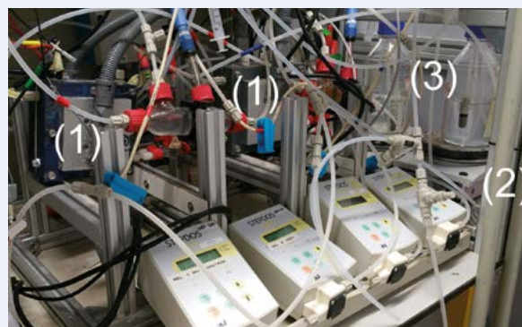
Figure 3: Bio-electrochemical ammonium recovery setup with microbial electrolysis cells (1), trans membrane chemisorption units (2) and acidic ammonium recovery solutions (3). [2]
