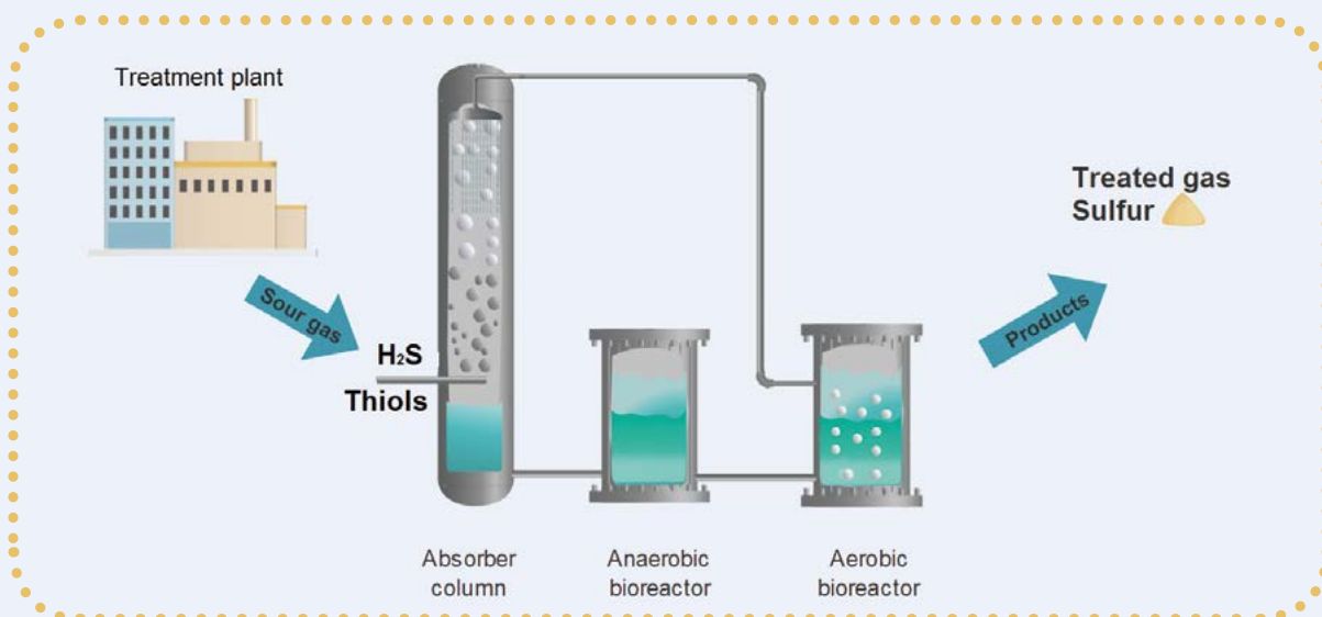
Research graphical abstract with a newly proposed line-up for hydrogen sulfide removal in the presence of thiols
