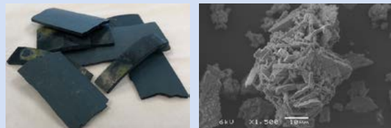
Fig. 2 Image of a vivianite sample from an STP and SEM image of a vivianite particle recovered from digested sludge.
