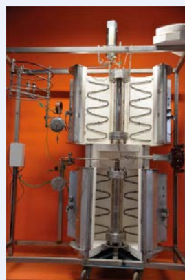
Fig 3a. SCWD Pilot plant (5 kg/h Brine)
