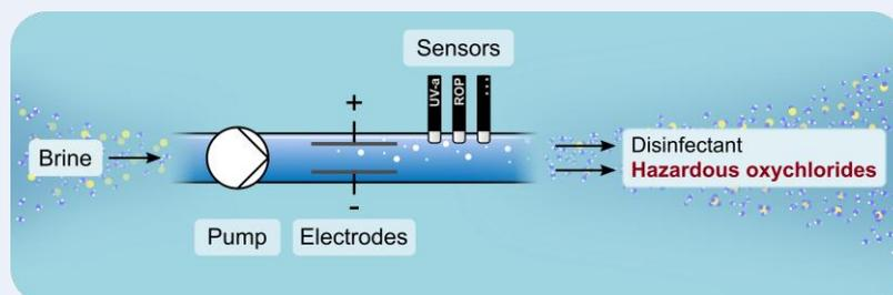
The goal of this project is to increase our understanding of electrochlorination, specifically how process parameters impact sensor data. This information is imperative to improve the prediction of chlorate and perchlorate formation.
