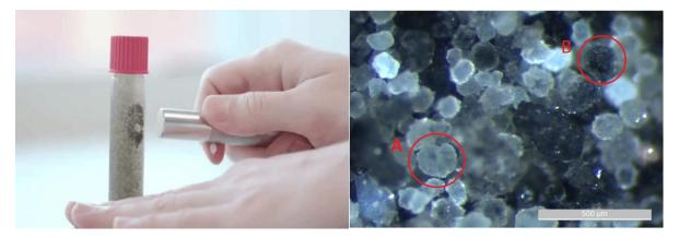
**Figure 1: (Left):** Vivianite concentrates from sludge getting attracted to a magnet. **(Right)** Vivianite crystals separated from sludge as viewed under a light microscope (scale bar 500  $\mu$ m). The darker blue colors (inset B as compared to inset A) indicate a higher extent of oxidized Fe in the sample.
