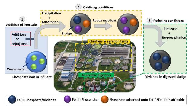
**Figure 2: Vivianite as an important P sink -** The picture shows a wastewater treatment plant (WWTP) and the insets show the type of interactions between Fe and P at different stages of the WWTP. Regardless of whether Fe(II) or Fe(III) ions are added, most of the P bound to Fe is transformed into vivianite in the anaerobic digestion tanks.
