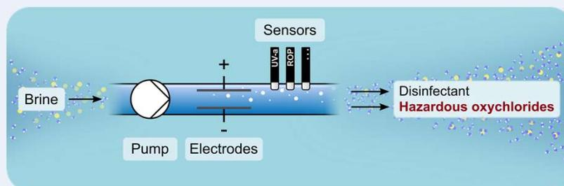
Impedance measurements could yield valuable information about the reactions taking place at the electrodes which, when combined with a model, could form a robust monitoring solution.
