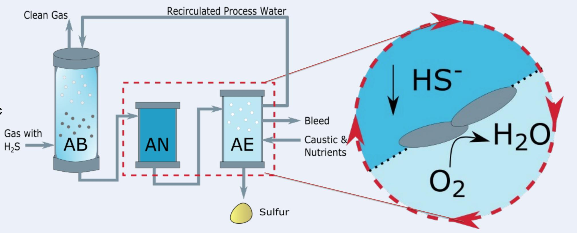
Fig 1. Current process design for the biodesulfurization process with an absorber column (AB), anaerobic reactor (AN), followed by the aerobic reactor (AE). The shuttling capacity occurs between the AN and AE reactors where the bacteria remove the HS<sup>-</sup>, reduce oxygen, and produce elemental sulfur.
