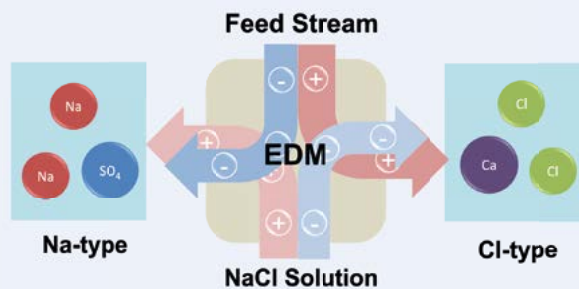
Fig 1 . Desalination with EDM: divalent ions from feed stream rearrange with monovalent ions from NaCl solution
