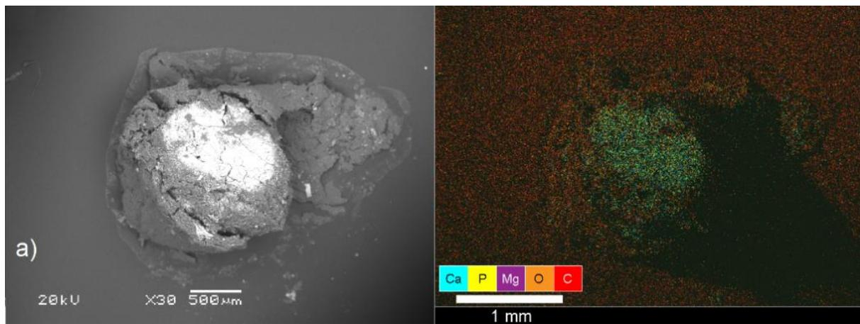
Figure 1, Scanning electron microscope (SEM, left) and electron dispersive x-ray (EDX, right) images of a calcium phosphate granule with an inorganic core consisting of calcium phosphate (EDX green) (Cunha et al. 2018).
