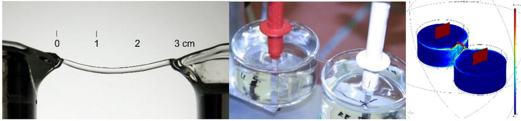
Fig. 1 – EHD liquid bridge. Left: bridge; middle: bridge with set-up; right: E-field 3D simulation
