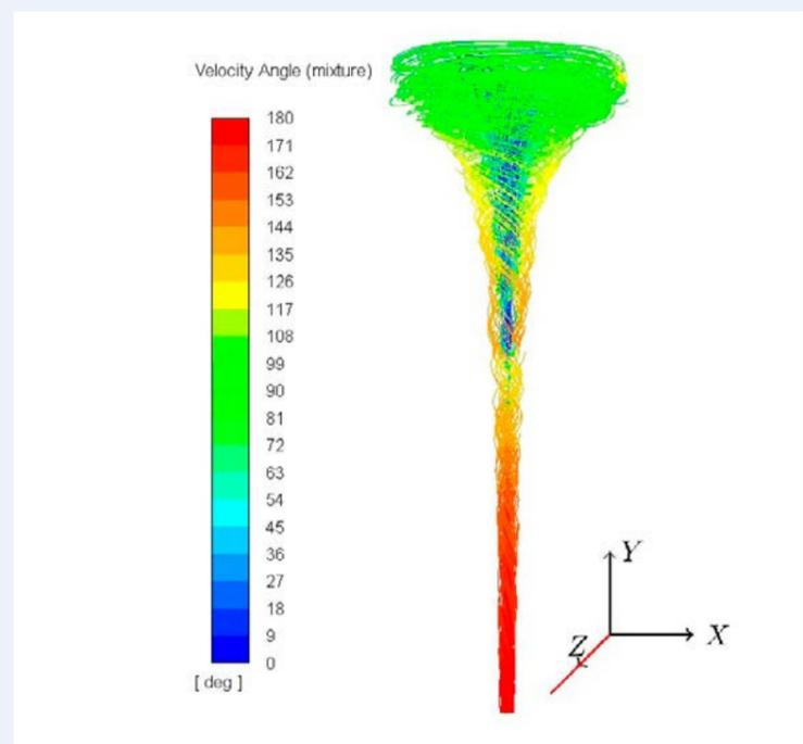
Fig 3. ANSYS Simulation result for velocity angle in degrees between flowlines and y-axis.
