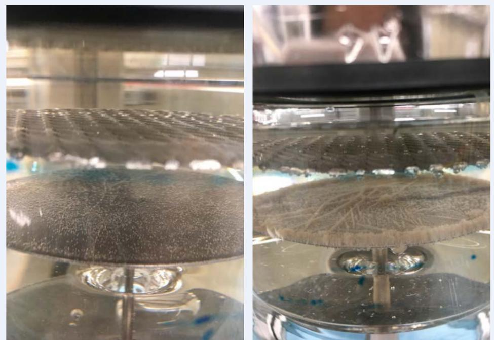
Figure 4. The surface of Ti cathode are totally covered by calcium phosphate precipitates after 24 hours' electrolysis. Conditions: 20 mA; 1.0 Ca<sup>2+</sup>, 0.6 mM HPO<sub>4</sub><sup>-</sup>.
