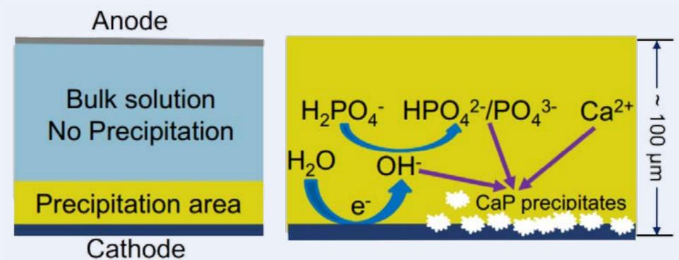
Figure 3. Mechanism of electrochemical induced calcium phosphate precipitation.
