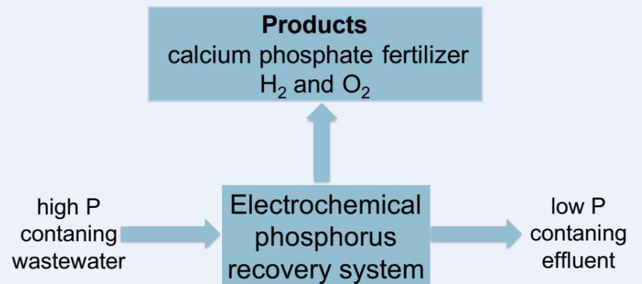
Figure 2. General overview of the electrochemical P recovery system.
