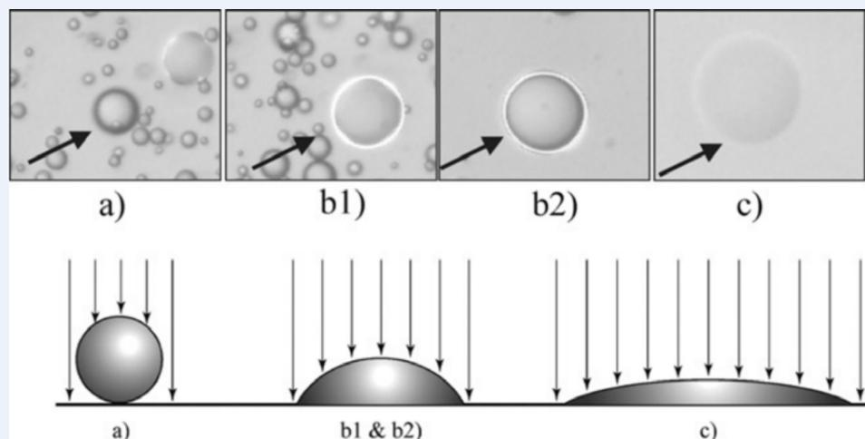
Figure 3: Microscopic appearances of a) an adhered droplet, b1 & b2) spread droplets with different contact angles, c) spread droplet with low contact angle (figures from [2]).
