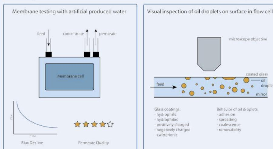
The appearance of the oil droplets in the flow cell changes with adhesion and spreading, thus allowing us to study the interaction of the emulsion with the different surface chemistries (Figure 1).
