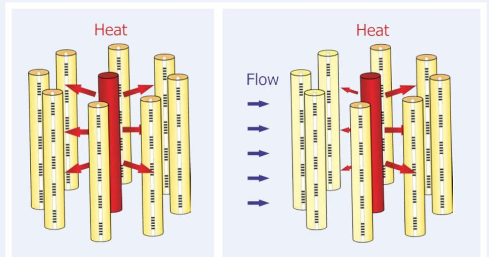
Fig. 3: Principle of FBG flow sensor. Without the presence of flow, all fibers should detect the same temperature if placed at the same distance from the heating fiber. Introducing flow from the left side will make the temperature on the left side lower than on the right.
