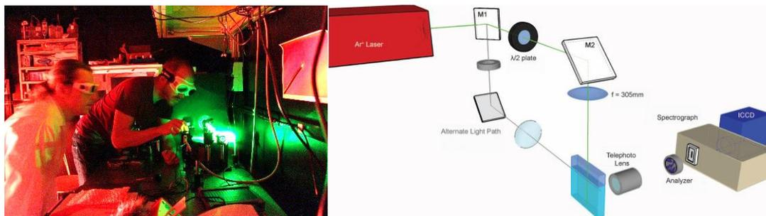
Fig. 1: Wetsus Optical Metrology Lab (snapshot, left); Diagram of a imaging Raman spectrometer<sup>1</sup>
