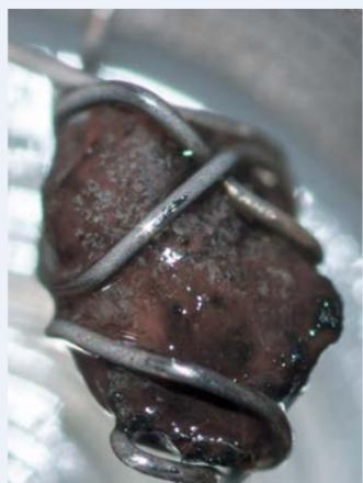
Fig. 1a: Single AC granule with partial biofilm growth and coiled with platinum wire [4].
