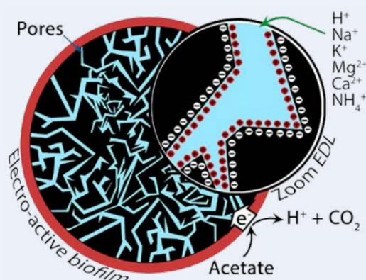
Fig. 1b: Acetate conversion and storage of electrons within AC granules via EDL formation [4].
