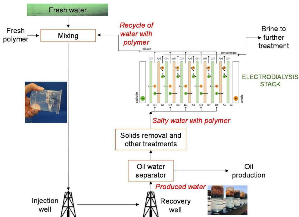
Figure 1. Scheme of the use of electrodialysis for the recovery of polymeric solutions from EOR
