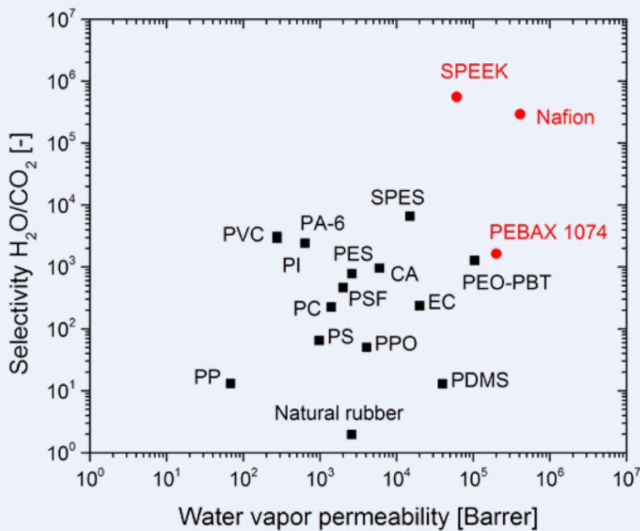
Figure 1: Water vapor permeability and water vapor/CO<sub>2</sub> selectivity for various polymers. SPEEK, Nafion® and PEBAX® 1074 show exceptionally high water vapor/CO<sub>2</sub> selectivities and water vapor permeabilities and are therefore considered for further investigations. [S. Metz "Water vapor and gas transport through polymeric membranes", University of Twente, 2003; and other sources]
