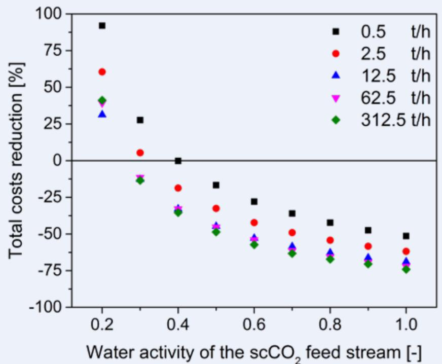
Figure 2: The total costs reduction of the membrane based process relative to the total costs of the zeolite process as a function of the feed stream water activity. At water activities above 0.4, the membrane based process becomes more cost efficient than the commercially used zeolite based process.
